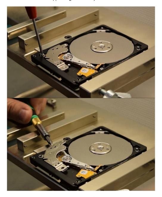
Picture 5.5. Removing the magnet
