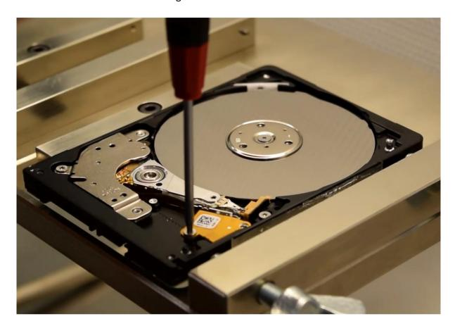
Picture 5.3. Removing the flat cable
