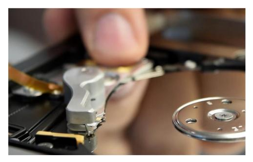
Picture 5.8. Moving the heads over the platters
