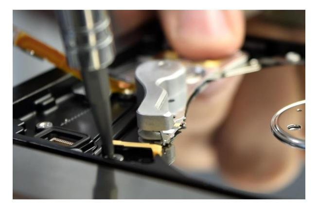
Picture 5.15. Mounting the ramp
