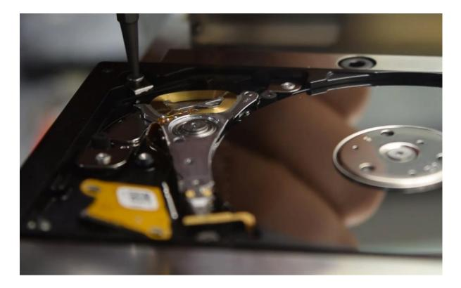
Picture 5.17. Removing the screw from the bottom magnet
