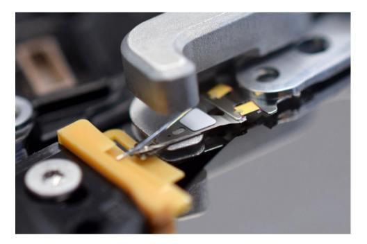
When the tool is mounted, gently move the heads over the platters and stop when the ramp is free for dismounting.
