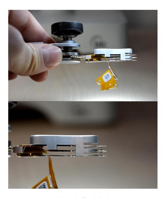
Picture 5.13. Lifting the heads
