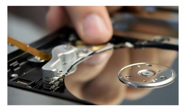
Picture 5.10. Sliding the heads off the platters
