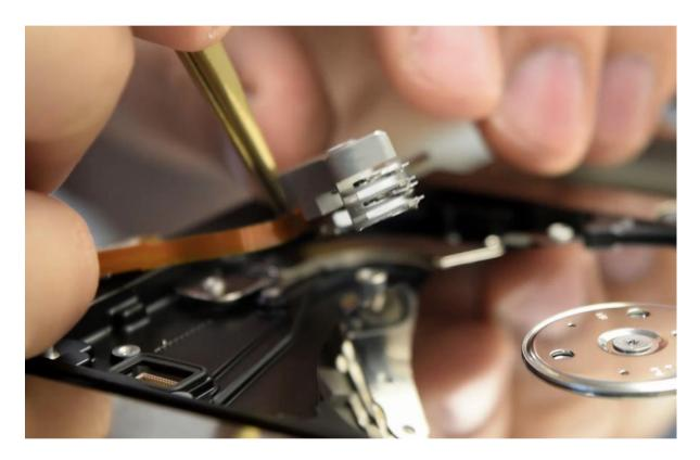
Picture 5.12. Lifting the heads
