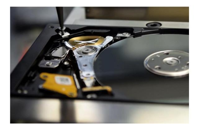
Picture 5.6. Tightening the bottom magnet
