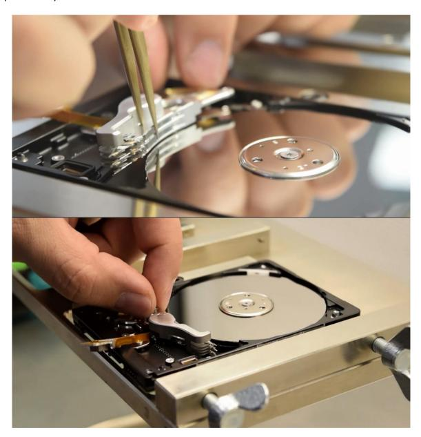
Picture 5.14. Positioning the head stack assembly
