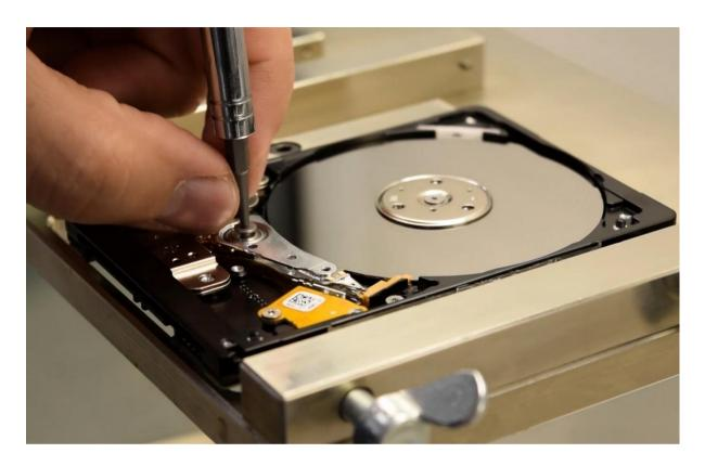
Picture 5.18. Removing the screw from the HSA
